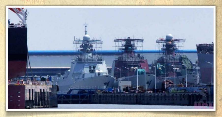
The 3<sup>rd</sup> generation Type 052D guided missile destroyer on the left was launched in 2014. The other two will be launched in 2015. There are five other Type 052Ds under construction. The Type 052D has 64 vertical launched cells, each with 1 to 4 missiles. It carries the YJ-12 anti-ship missile with 400 KM range. China plans to deploy 10 Type 052D destroyers. China has already 6 Type 051 and Type 052A/B/C destroyers.
